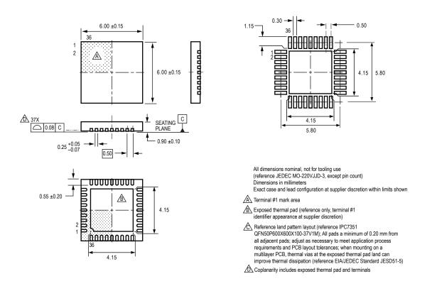
EV Package, 36-Pin QFN with Exposed Thermal Pad
