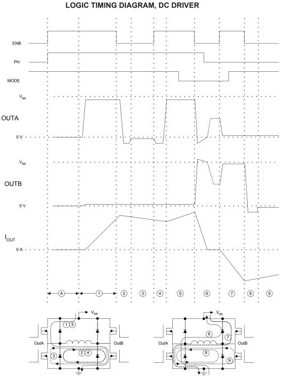
(A) Charge Pump and VREG Power-up Delay (≈200 μs)
