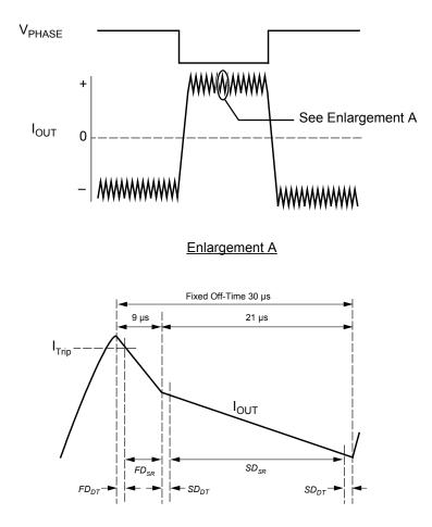
Figure 2: Mixed Decay Mode Operation
