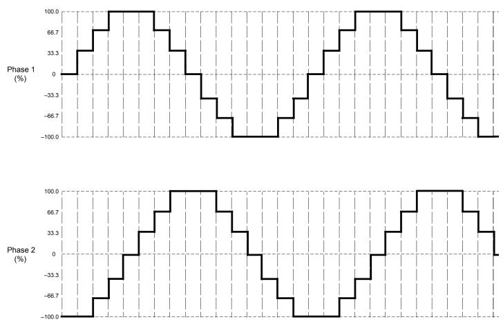
Figure 5: Decay Modes for Quarter-Step Increments
