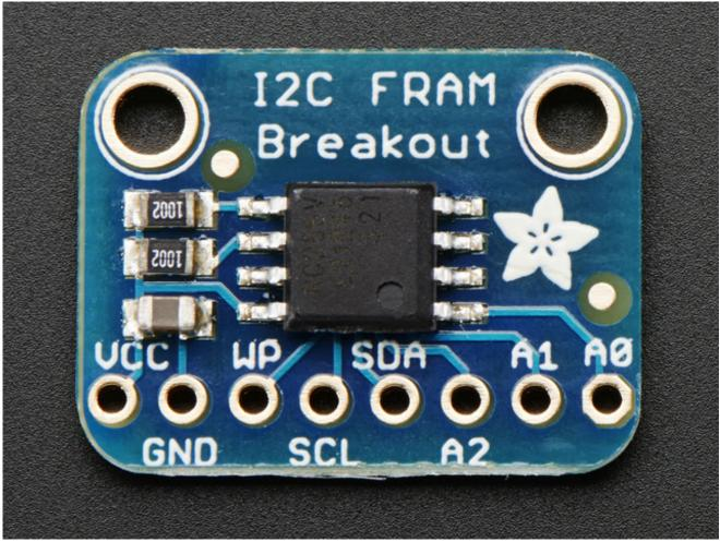
You can easily wire this breakout to any microcontroller, we'll be using an Arduino
