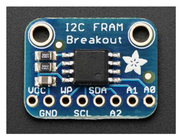
The FRAM chip is the little guy in the middle. On the bottom we have the power and interface pins
