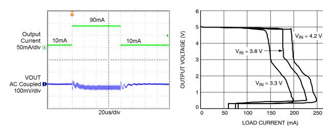
Figure 12. Load Transient Response
