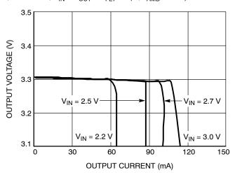
Figure 14. Output Voltage vs. Input Voltage
