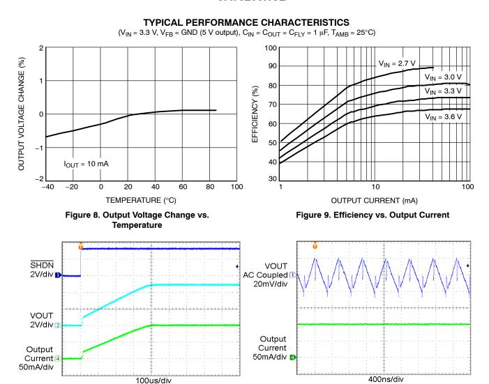
Figure 10. Power Up Waveform  $(I_{OUT} = 100 \text{ mA})$
