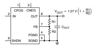
Figure 20. Programming the Adjustable Output
