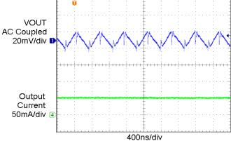
Figure 18. Power Up Waveform  $(I_{OUT} = 50 \text{ mA})$
