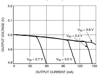
Figure 4. Output Voltage vs. Input Voltage
