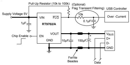
**Note:** A low-ESR 150 $\mu$ F aluminum electrolytic or tantalum between V<sub>OUT</sub> and GND is strongly recommended to meet the 330mV maximum droop requirement in the hub V<sub>BUS</sub>. (see Application Information Section for further details)
