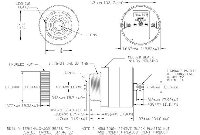
OTE B: MOUNTING- REMOVE BLACK PLASTIC NUT AND INSERT THREADED FRONT THROUGH 1.25" HOLE PUNCHED IN PANEL, IF ORIENTATION IS NEEDED, NOTE LOCKING FLATS ON DRAWING, SCREW NUT BACK ON. DO NOT OVERTIGHTEN.
