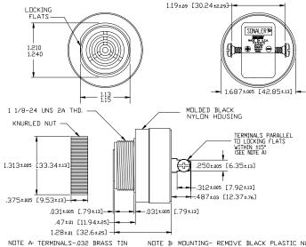
NOTE A: TERMINALS-032 BRASS TIN PLATED, TAPPED FOR #6-32 SCREW. TWO #6-32 NICKEL PLATED BRASS SCREWS INCLUBED. VILL ACCEPT 1/4' QUICK CONNECT. B: MOUNTING- REMOVE BLACK PLASTIC NUT AND INSERT THREADED FRONT THROUGH 1.25' HOLE PUNCHED IN PANEL, IF DRIENTATION IS NEEDED, NOTE LOCKING FLATS ON DRAWING SCREW NUT BACK ON. DO NOT OVERTIGHTEN.
