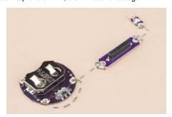
With new thread once again, sew down the negative pin of the LED, stitch down to the negative side of the battery pack, and sew down both negative sew taps, again stitching around the board to connect them rather than in a straight line across the board. This prevents the battery from sitting on top of the connecting thread, which could cause a short circuit.
