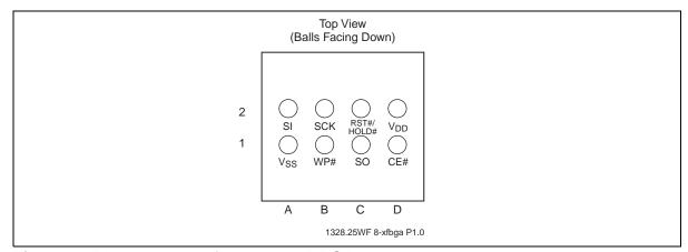
Figure 3: Pin Assignment for 8-bump XFBGA
