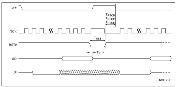
Figure 5: Reset Timing Diagram
