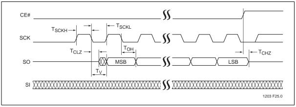
Figure 28:Serial Output Timing Diagram
