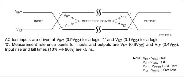
Figure 30:AC Input/Output Reference Waveforms
