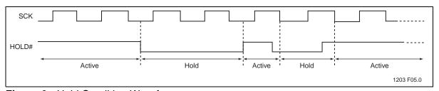
Figure 6: Hold Condition Waveform
