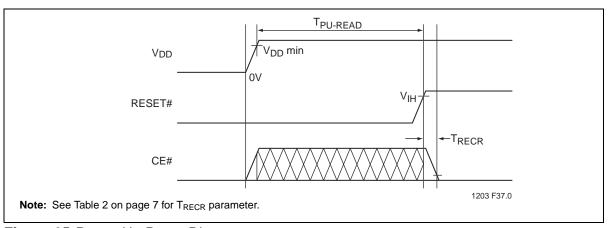
Figure 25: Power-Up Reset Diagram
