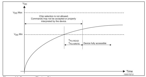
Figure 26: Power-up Timing Diagram
