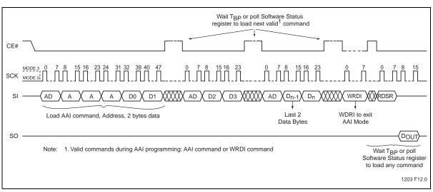
Figure 13: Auto Address Increment (AAI) Word Program Sequence with Software End-of-Write Detection
