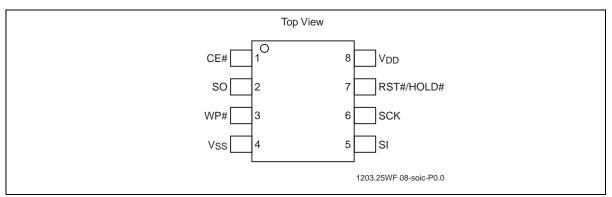
Figure 2: Pin Assignment for 8-Lead SOIC
