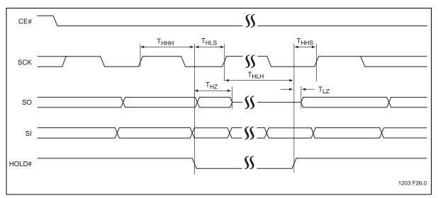
Figure 29: Hold Timing Diagram
