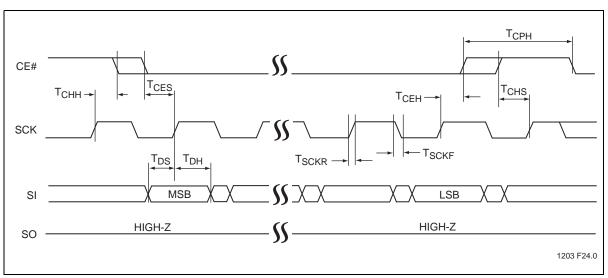
Figure 27: Serial Input Timing Diagram
