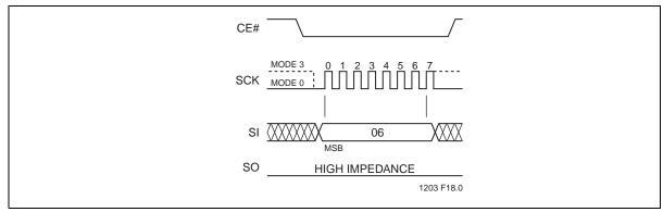
Figure 19: Write Enable (WREN) Sequence
