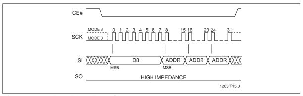
Figure 16:64-KByte Block-Erase Sequence
