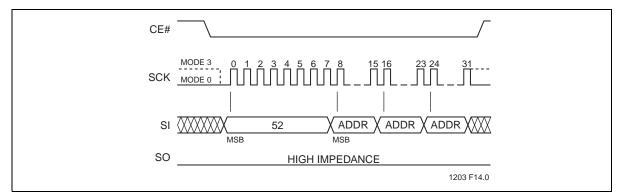
Figure 15:32-KByte Block-Erase Sequence
