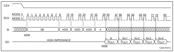
Figure 8: High-Speed-Read Sequence
