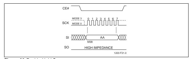
Figure 22: Enable-Hold Sequence
